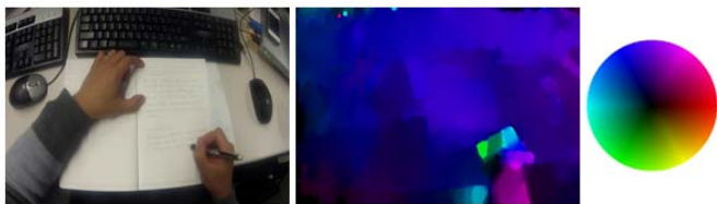
Fig. 6. Optical flow (middle) of egocentric video (left). Note the diverse motion in the hand region. Color map for flow visualization is shown in the rightmost.
