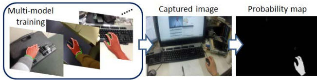
Fig. 4. Hand segmentation using multimodel hand detector.
